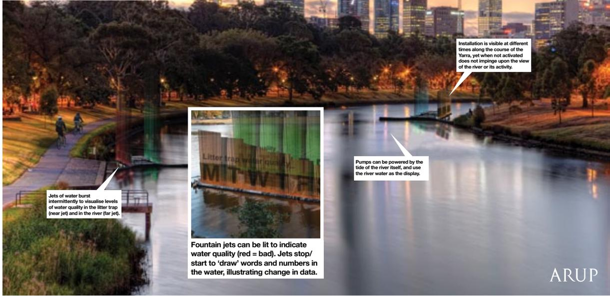
Jets of water burst intermittently to visualise levels of water quality in the litter trap (near jet) and in the river (far jet).
